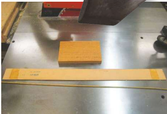
▲ Pic.1 Dominic used an offcut of iroko for the knife's handle and a brass rod he had from another project
